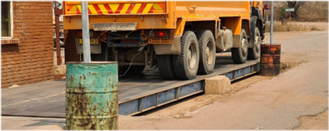
Figure 12: Open Side of Weighbridge
